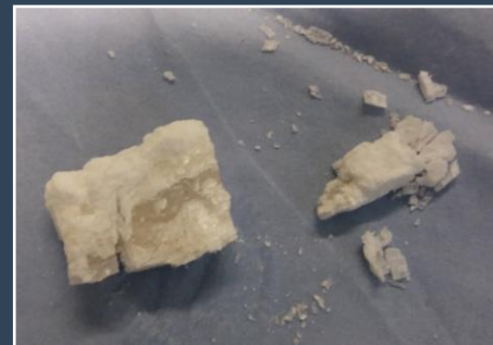
Fig. 1: Severe calcite efflorescence from exposure to acetic acid. The specimen also depicts extensive fracturing which led to decrepitation.
