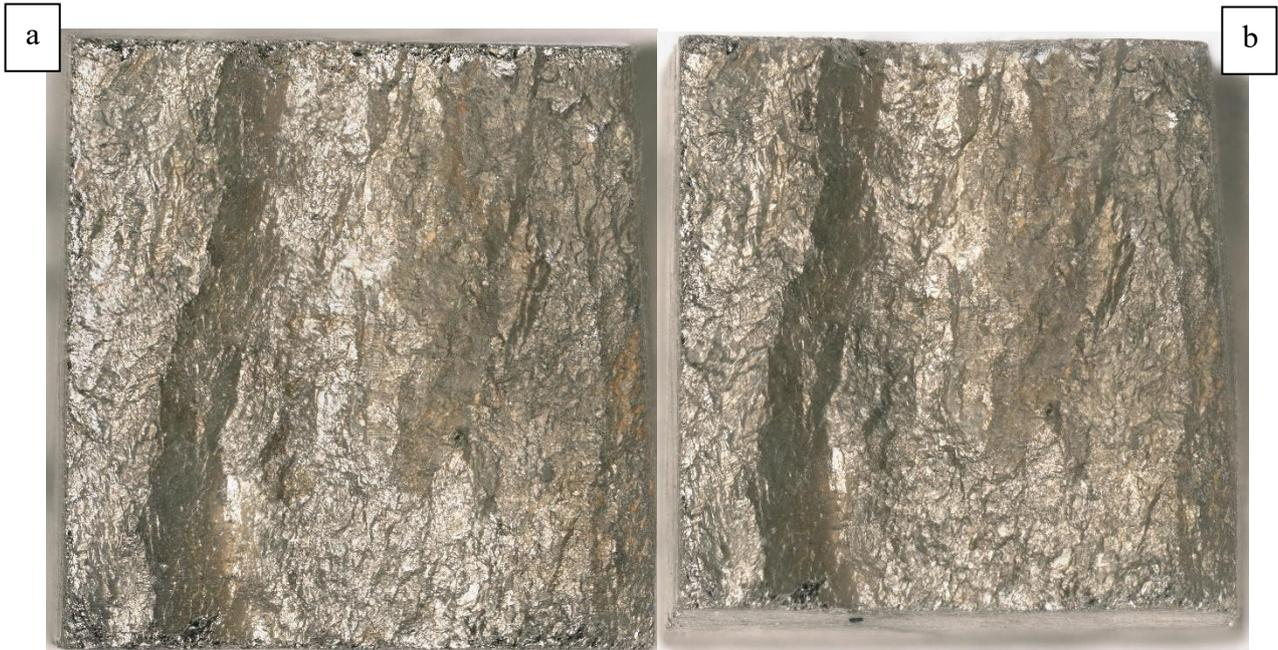
*Figure 3. Pyrite sample 1 (50x magnification) a.) before & b.) after experimentation. The only visual difference is the duller appearance of the latter. Rusty oxidation products can be seen on the right side of the sample.*
