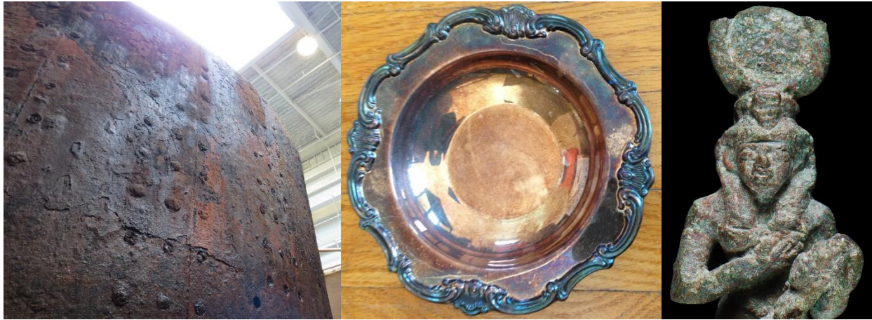
Figure 4. Images of three different metals corroding. These are all perceived differently based on the observer and the object's uses and values. 1) The USS Monitor's gun turret made of wrought iron (Newport News, VA, USA). 2) A silver dish with iridescent tarnish. 3) A copper alloy statuette of Isis suckling Horus from the Bristol Museum (UK).
